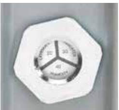
HUMIDITY INDICATOR Indicates 20%, 30%, and 40% relative humidity ranges. Colour changes when inside humidity exceeds the indicated level. Resets as humidity decreases; used along with PRV.
