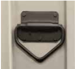
LIFT / TIE DOWN RINGS 2" (50 mm) diameter lift grips, spring loaded, pivot 180°, (340kg/ring rating installed). (453 kg/ring rating). Plated Steel and Black Stainless Steel.
