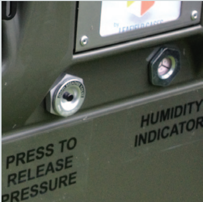
Pressure equalisation valves and humidity indicators
